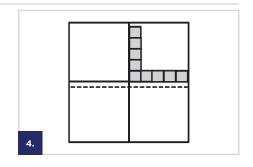
Install the Tiles: Lay Attraxion pieces from the center of the room in a pyramid fashion while working towards the walls as shown in Figure 5. Ensure that the pattern is always aligned with the starting line. Measure, mark and cut perimeter pieces maintaining a  $\frac{1}{4}$ " expansion space at all fixed vertical objects.
